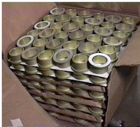
FIGURE 2 - Parts are singled layered and divided with corrugated pads.
