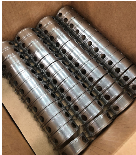
FIGURE 3 - Parts can be layered in rows and divided by corrugated pads.
