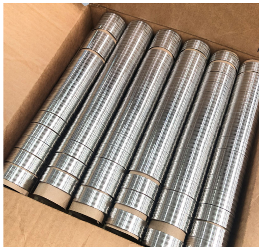
FIGURE 4 - Round parts can be slid through a tightly rolled up divider.
