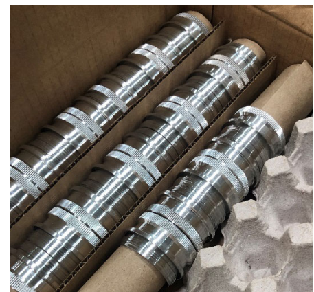
FIGURE 9 - Parts are secured using a rolled up divider with a divider between the tubes.
