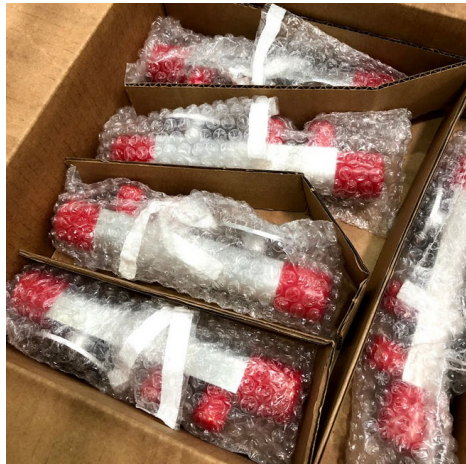
FIGURE 10 - Parts can be segregated with the use of dividers to ensure critical surfaces are not damaged, caps are used.
