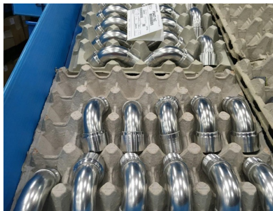
FIGURE 8 - Flanged FS's are packed securely in egg trays.
