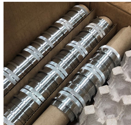
FIGURE 6 - Parts are secured using a rolled up divider with a divider between the tubes.
