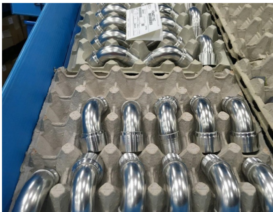
FIGURE 5 - Flanged FS's are packed securely in egg trays.
