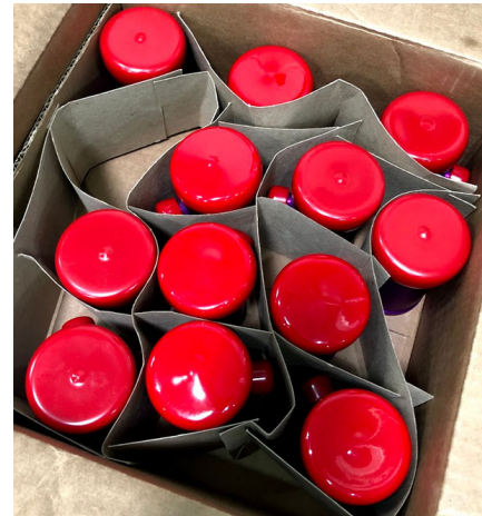
FIGURE 10 - Parts can be segregated with the use of dividers to ensure critical surfaces are not damaged, caps are used.
