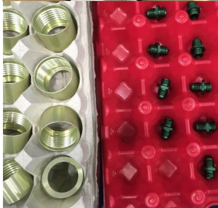
FIGURE 7 - Parts are packed in egg trays
