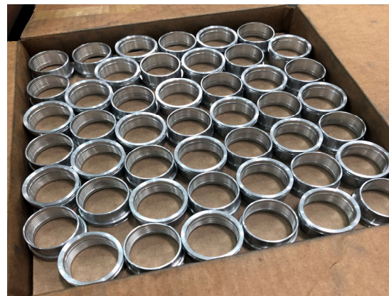
FIGURE 2 - Parts are singled layered and divided with corrugated pads.
