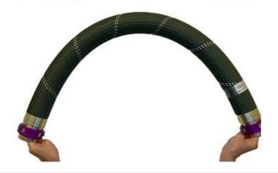
Hydraflow's HS58-32 hose has a smooth bore silicone inner line with a Nomex® outerbraid. The HS58-32 hose is flexible and lightweight, making it ideal for vacuum waste and coolant applications with tight installation tolerances.
