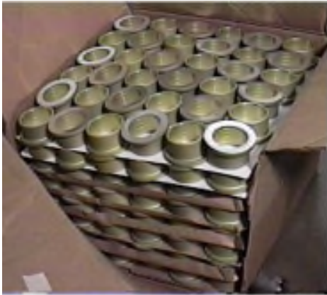
FIGURE 2 - Parts single layered and divided by corrugated pads.
