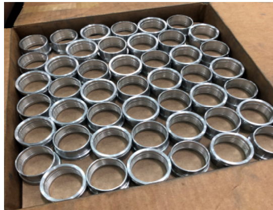
FIGURE 2 - Parts single layered and divided by corrugated pads.
