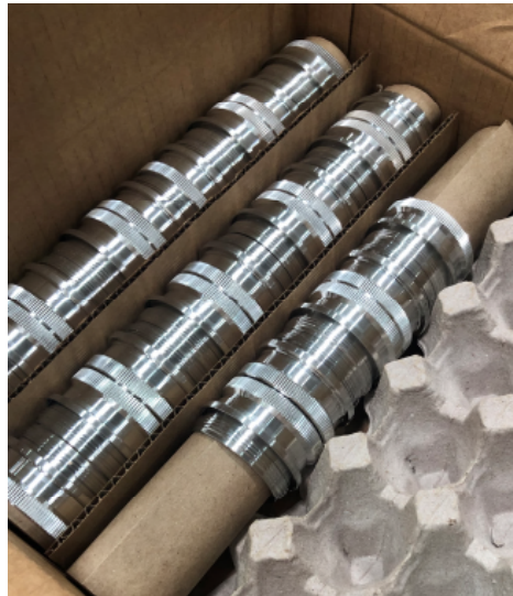
FIGURE 7 - Parts are layered and divided by columns using corrugated pads or dividers.
