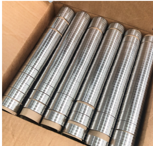
FIGURE 5 - Circular parts are slid through a rolled up divider.
